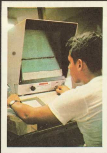
The Recordak Lodestar Reader—Resupply items, stock numbers, locations and other important data are kept on microfilm for quick reference by Headquarters and A Company personnel.
